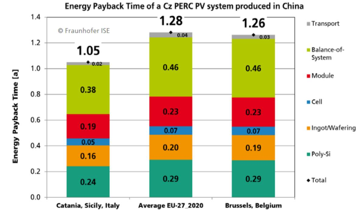
A typical PV system will give back the energy required for **fabrication in 1 year in CH** Module around 60-65% of the total.
